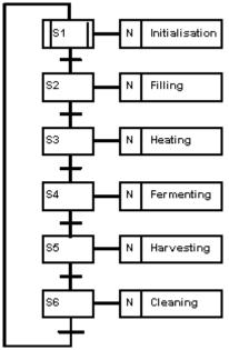
We start at the top with the Initialization: since we do not know the status of the system when we first switch it on, we must check the position of the valves, etc. Then we start filling till the right level has been reached.
