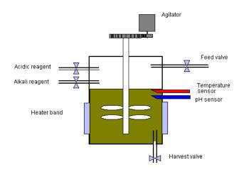
All external interfaces are defined here (step 1). There is a large vessel, which can be filled (Feed Valve) with the liquid, can be heated with the heater band (cooling via convection), can be stirred via the motor, and where acid and alkali fluid can be added into the vessel.
