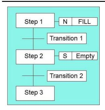
SFC supports alternative sequences and parallel sequences, such as commonly required in batch applications. For instance, one sequence is used for the primary process, and a second for monitoring the overall operating constraints. And this occurs within the same overview and structure.
