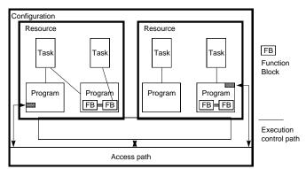
At the highest level, the entire system required to solve a particular control problem can be formulated as a *Configuration*, including the arrangement of the hardware, memory addresses for I/O channels and system capabilities.
