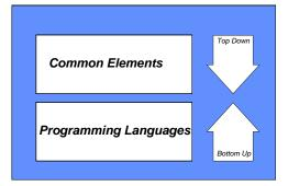
Also, the standard allows two ways of developing your program: top down and bottom up. Either you specify your whole application and divide it into sub parts, declare your variables, and so on. Or you start programming your application at the bottom, for instance via derived functions and function blocks. Whichever you choose, the development environment will help you through the whole process.
