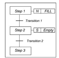
SFC describes graphically the sequential behavior of a control program. With this it structures the internal organization of a program, and helps to decompose a control problem into manageable parts, while maintaining the overview.
