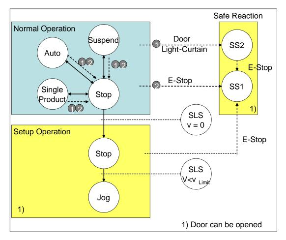
For the emergency stop functionality, we want one switch for the whole machine. We need to connect the status of this knob (On or Off) to the application. Also, we need to restart the machine after releasing and acknowledging the emergency button.
