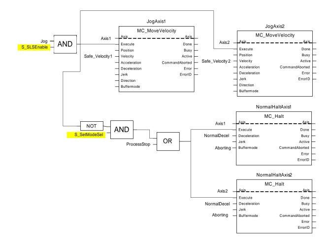
MC\_Halt is used here because the halting mode can be aborted by another command, which in case of MC\_Stop not the case is.
